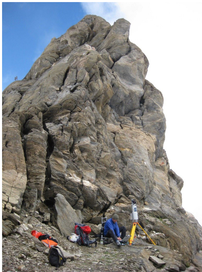
Figure 4: Terrestrial Laserscanning below the Magnetköpfl (© Ingo Hartmeyer)
