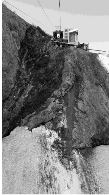
Figure 1: Permafrost related rock fall at the Kitzsteinhorn at approx. 2950 m (August 18, 2012 at 3pm). At the slip surface ice became visible after the failure. The Kitzsteinhorn region is one of our six test sites. Photo taken by M. Keuschnig.
