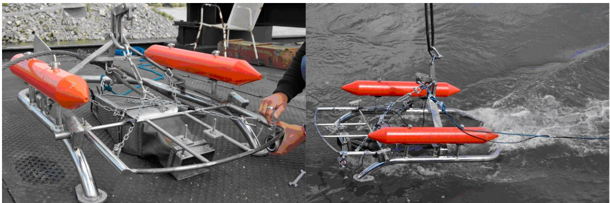
Figure 3: Adapted Basket sampler (based on the sampler of BfG, Koblenz, Germany).
