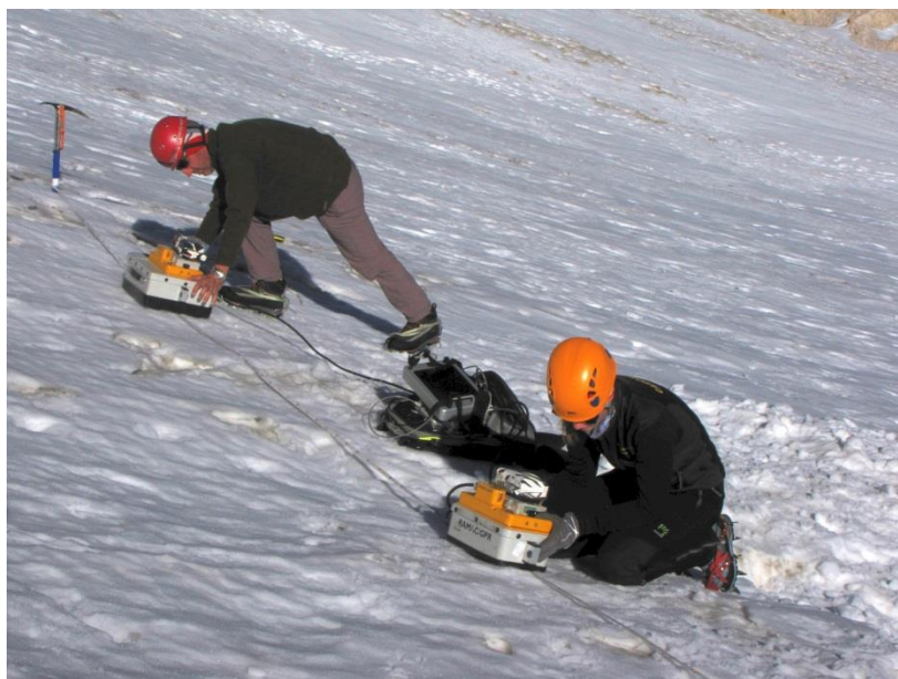
Figure 3: In 2013, ground-penetrating radar surveys of the glacier were performed. Photo: Matija Zorn.
