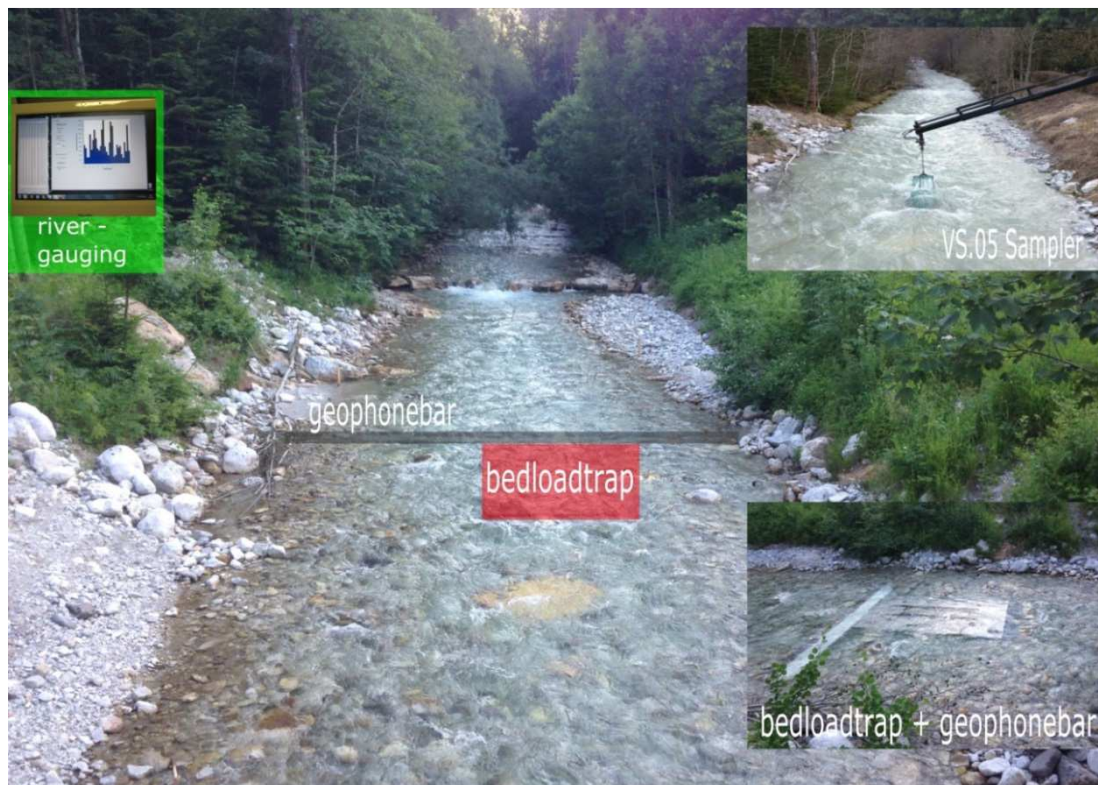
Figure 6.5: Arrangement of the integrative bedload monitoring system consisting of a bedload trap and a geophone bar ( center and lower right ) supported by a basket sampler ( upper right ). Bedload data acquisition and river gauging takes place in a monitoring station ( upper left ). Note: views in the center and the upper right are looking upstream.
