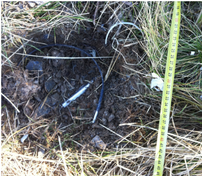
Figure 1.5.: The soil temperature logger on the Gscheideggkogel. With kind permission of the Nationalpark Gesäuse.
