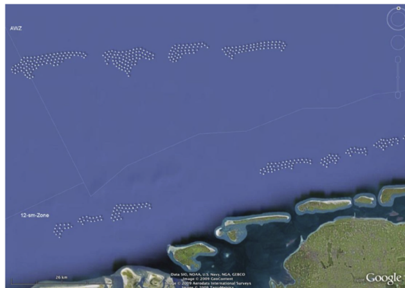
Fig. 4. An example for the North Sea wind farm designs was the “Island” solution. This design placed the wind turbines in such a way that they represented the old coastal line destroyed by a flood in early medieval times (Schöbel, 2011).
