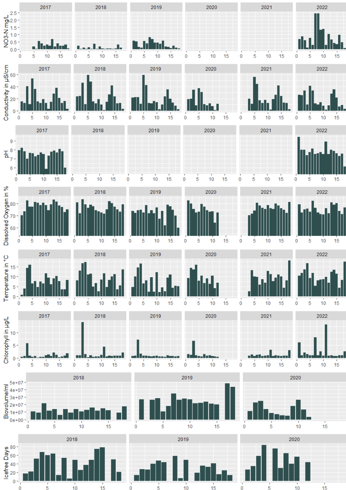
Figure 7 Shows the mean 2-meter values of the lakes. Biovolume was not evaluated in 2017 and the biovolume data of lake 2 in 2019 is missing. PH is missing in 2018-2021 and Nitrogen is missing in 2020 and 2021 due to problems with the sensor. Ice-free Days were calculated as the days between sampling and the lake temperature being above 2 °C and fluctuating. 2017 were no samples taken and no temperature logger data available. The lake "kleines Elend" was revisited in 2018 because on the regular date it was still covered in ice.
