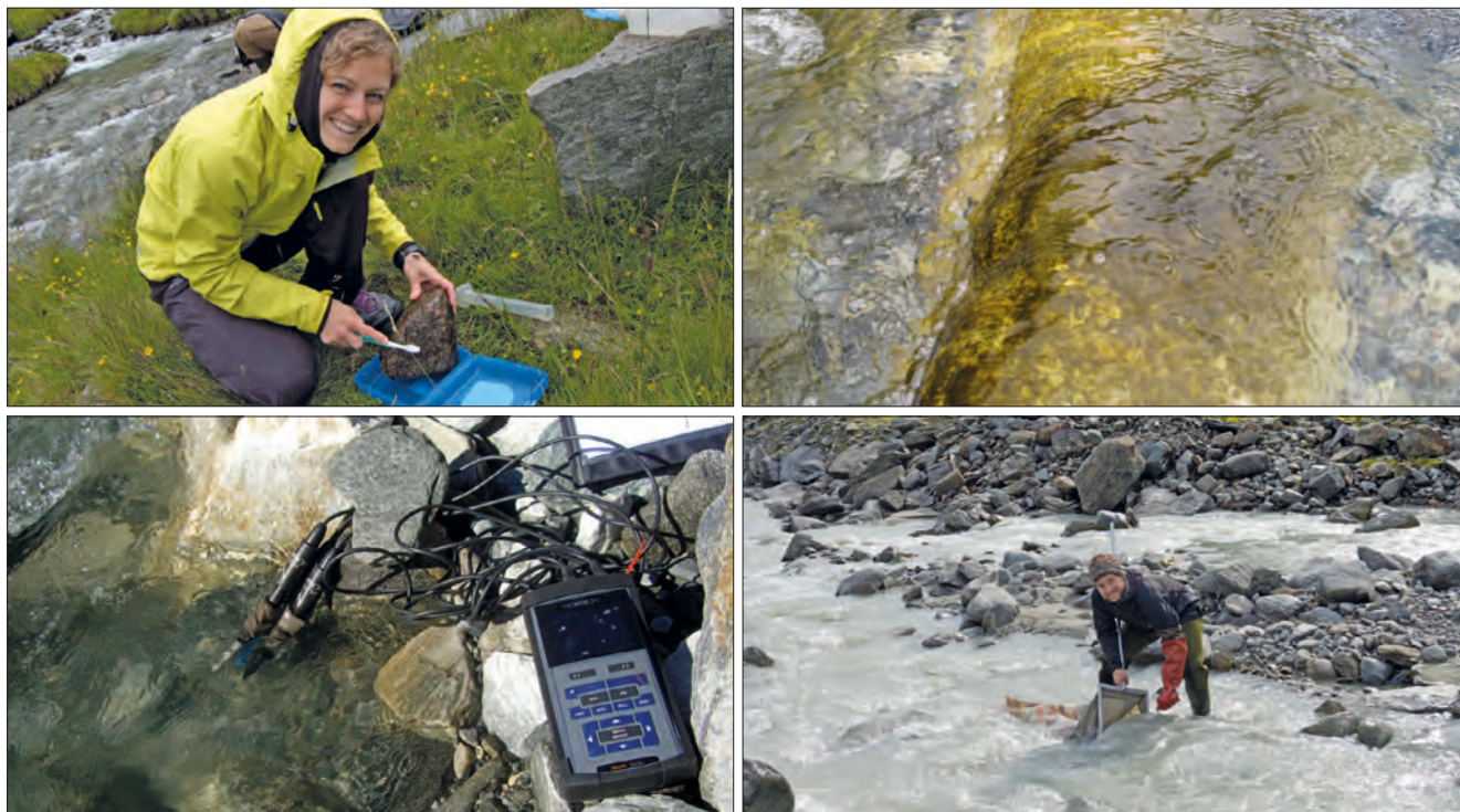
Top photos, from left to right: Taking a growth sample (photo: B. HECHENBLAICKNER), biofilm of the algae species Hydrurus (photo: G. NIEDRIST); bottom photos, from left to right: WTW MultiLine probe for measuring hydrochemical parameters (photo: G. NIEDRIST), taking samples of macrozoobenthos (photo: S. SCHÜTZ).
