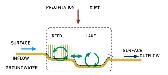
Figure 1. Scheme of inputs, outputs, and internal processes in Lake Neusiedl / Fertő. Source: Stalzer & Spatzierer (1987) (modified).
