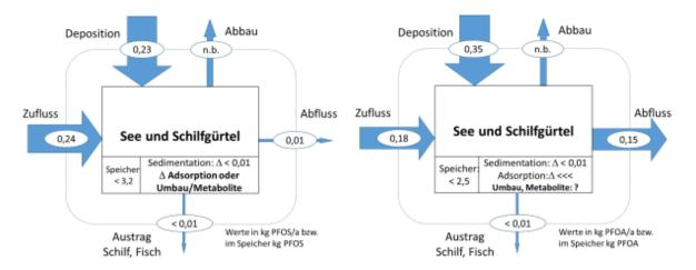
Figure 18. Estimation of a substance balance of the lake Neusiedl / Fertő (long term water balance combined with substance concentrations from 2017–2019) for PFOS (left) and PFOA (right)
