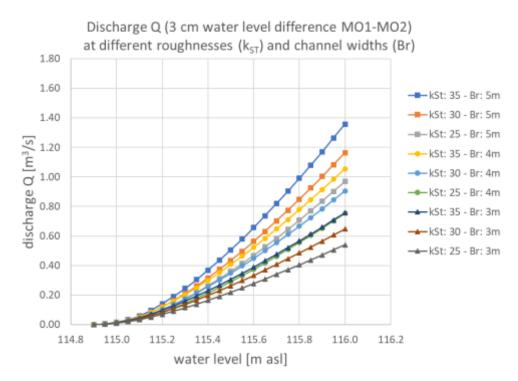
Figure 36. Relation between water level and discharge through a channel near Mörbisch assuming varying channel width, using the Manning-Strickler model (MO1 lake edge, MO2 reed belt).
