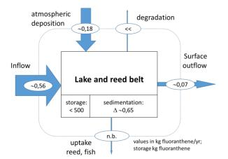
Figure 19. Estimation of a substance balance of the Lake Neusiedl / Fertő for fluoranthene (long term water balance combined with substance concentrations from 2017–2019).
