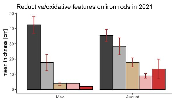
Figure 3: Bars represent mean thickness of reductive or oxidative features on iron rods for May and August. Bars are ordered from pure reductive features (black bar), mainly reductive (grey), transitional (brown), mainly oxidative (pink) to oxidative features (red)
