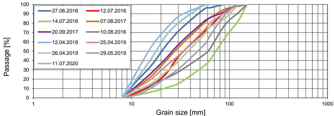
Figure 26 Grain size distribution  $>8\text{mm}$  derived by the basket sampler of the years 2016-2020, each measurement campaign consists of multiple single samples which were averaged for display.
