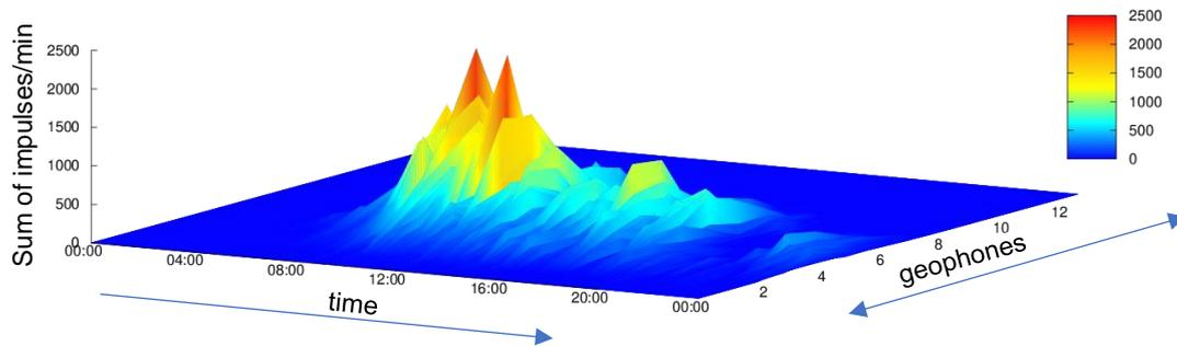
Figure 24: 24 hours geophone impulse graph of 08.07.2022 showing the temporal and special distribution, red indicates a high number of impulses per minute, blue indicates low impulses per minute.
