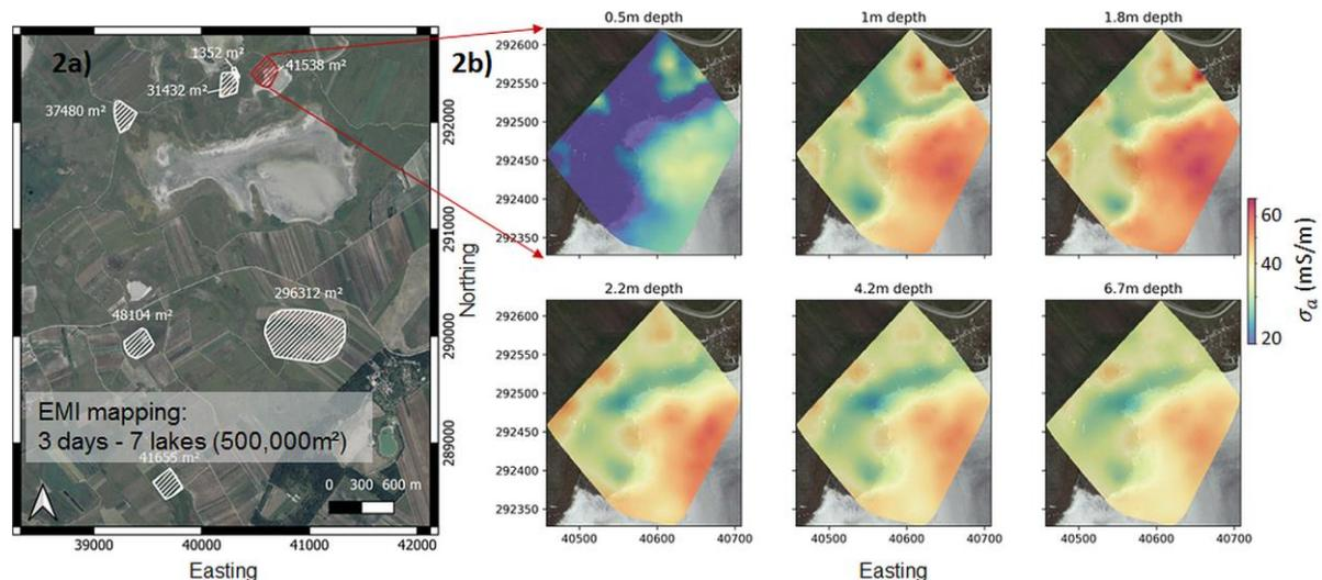
Figure 2: EMI measurements were conducted at different lakes covering a total area of 50 ha (Fig. 2a) to map variations in the apparent electrical conductivity ( $\sigma_a$ ). Illustrative results are presented in Fig 2b for a selected lake (red polygon in Fig. 2a) in terms of the lateral changes in  $\sigma_a$  sensed at different depths. The  $\sigma_a$  represents the average conductivity from the surface to the nominal depth of investigation
