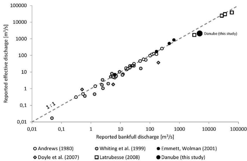
Figure 3: Effective discharge versus bankfull discharge for our study reach (Danube east of Vienna) and for comparison for other river reaches, data from literature [2, 10-12, 14], and modified from [15]
