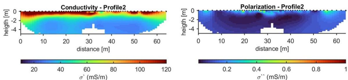
Figure 4: IP imaging results for data collected along Profiles 2 expressed in terms of the conductivity ( $\sigma'$ ) and polarization ( $\sigma''$ ). Blanked areas refer to model parameters of poor sensitivity.
