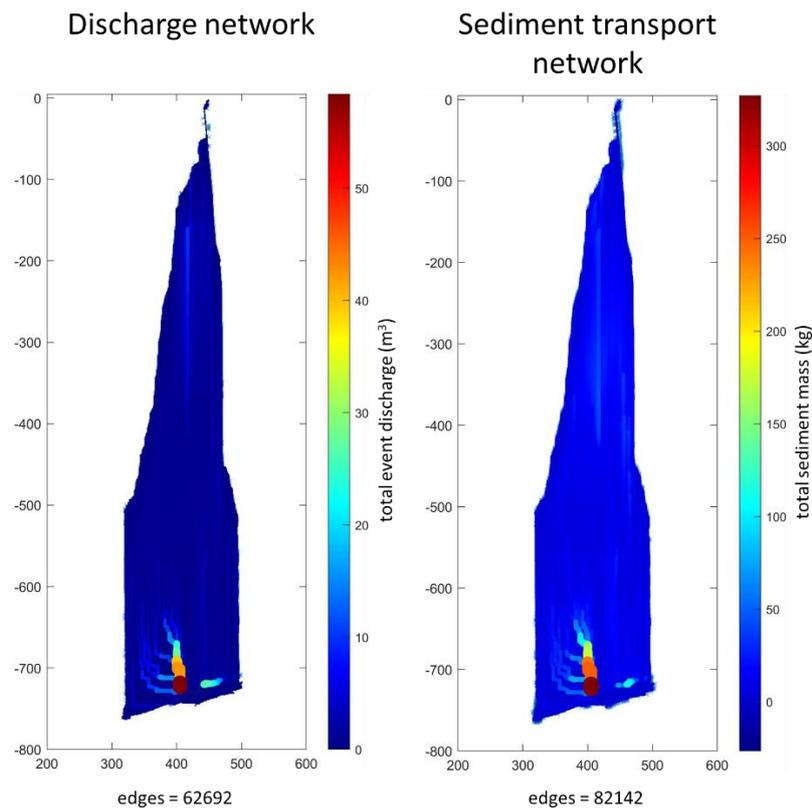
**Figure 1.** Discharge and sediment transport outputs from the MAHLERAN simulation represented as a network.
