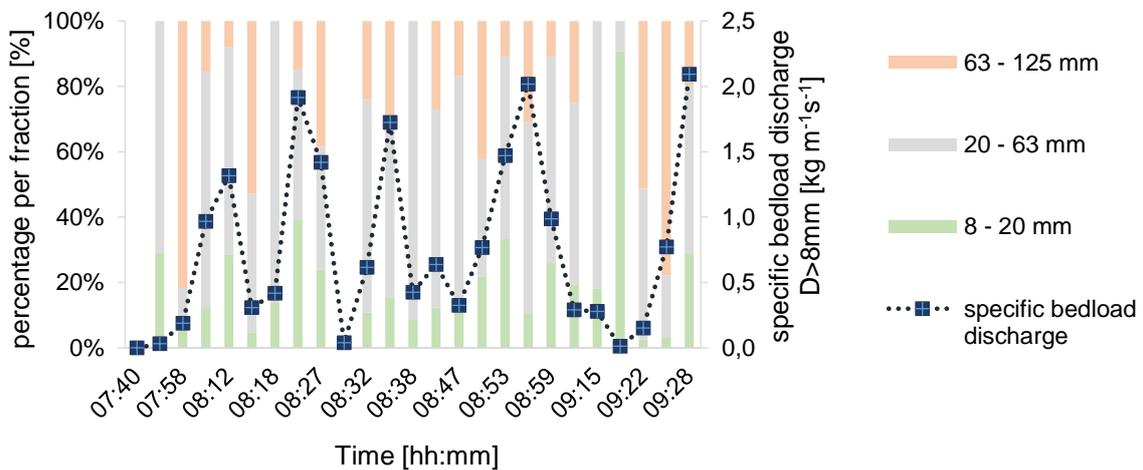
Figure 25: Grain size distribution during the event of 26.04.2019 derived from basket sampler D>8mm. the left vertical axis refers to the percentage per fraction displayed as a bar chart, the specific discharge is displayed as squares linked by a line and refers to the right vertical axis.
