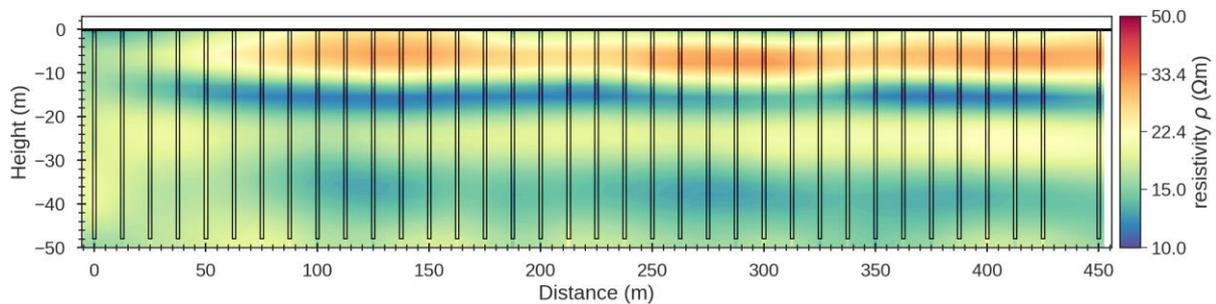
Figure 5: TEM imaging results presented in terms of the electrical resistivity ( $\rho$ ), the inverse from the conductivity ( $\rho = 1/\sigma$ ), to differentiate those from the EMI and IP. TEM soundings were collected in the area between Profiles 1 and 3.
