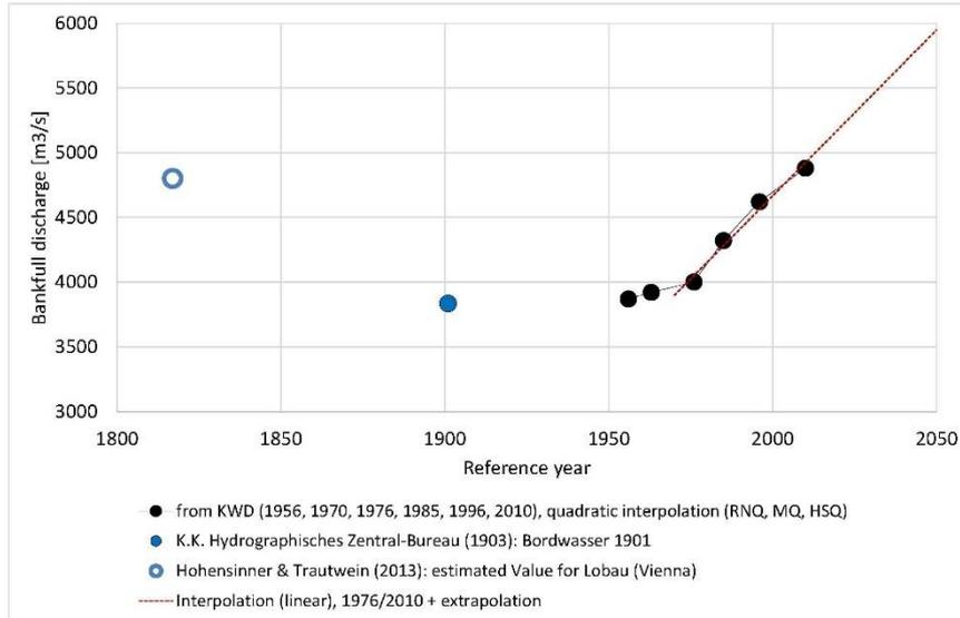
Figure 2: Bankfull discharges of the Danube east of Vienna, determined for the gauging station Hainburg, for different reference years (1817, 1901, 1956, 1970, 1976, 1985, 1995 and 2010); applying [26] and [29], and modified from [15]
