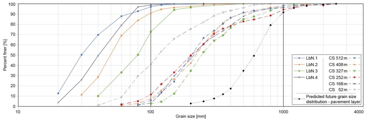
**Figure 17:** Partial grain size distribution curves: (a.) four line-by-number (LbN) analyses (continuous lines) and photogrammetric evaluations (dashed lines) for six characteristic points in the inaccessible canyon. (b.) the dotted black curve refers to the potential future grain size distribution of the pavement layer.
