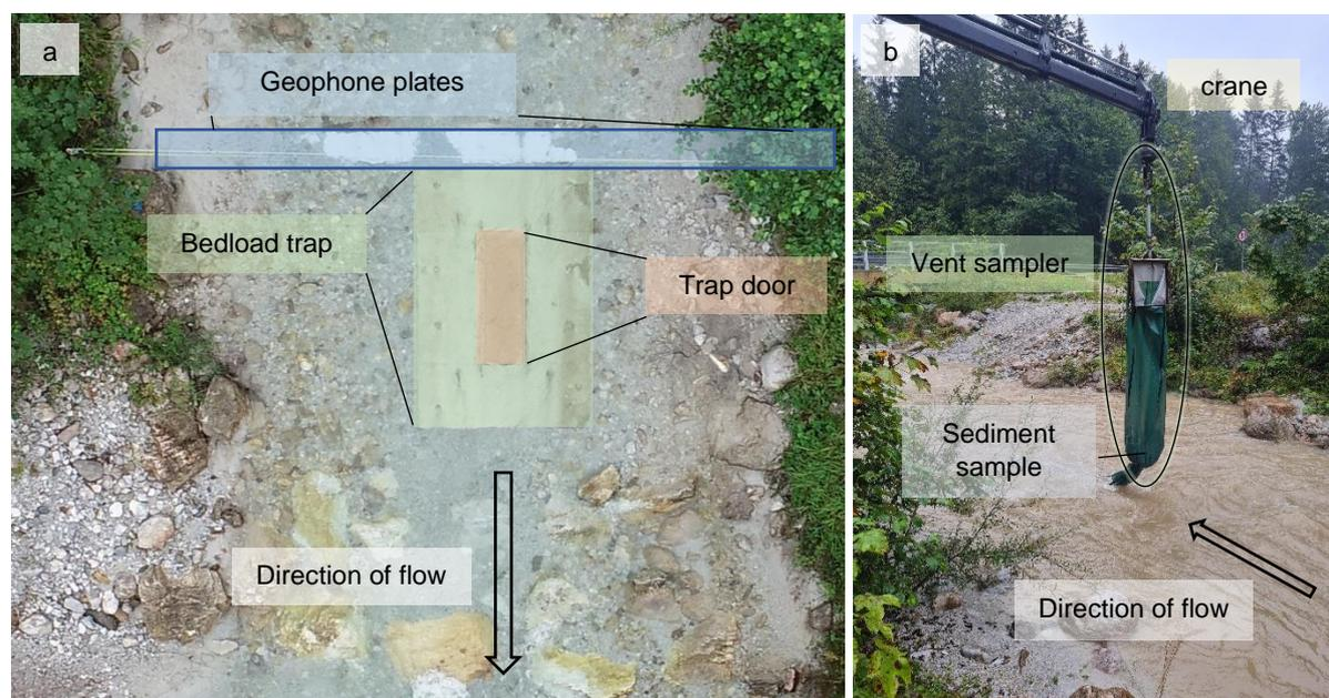
Figure 23: Integrative bedload monitoring at the Johnsbach stream: a) geophone pates and bedload trap (top few), b) vent sampler attached to crane with sediment sample.
