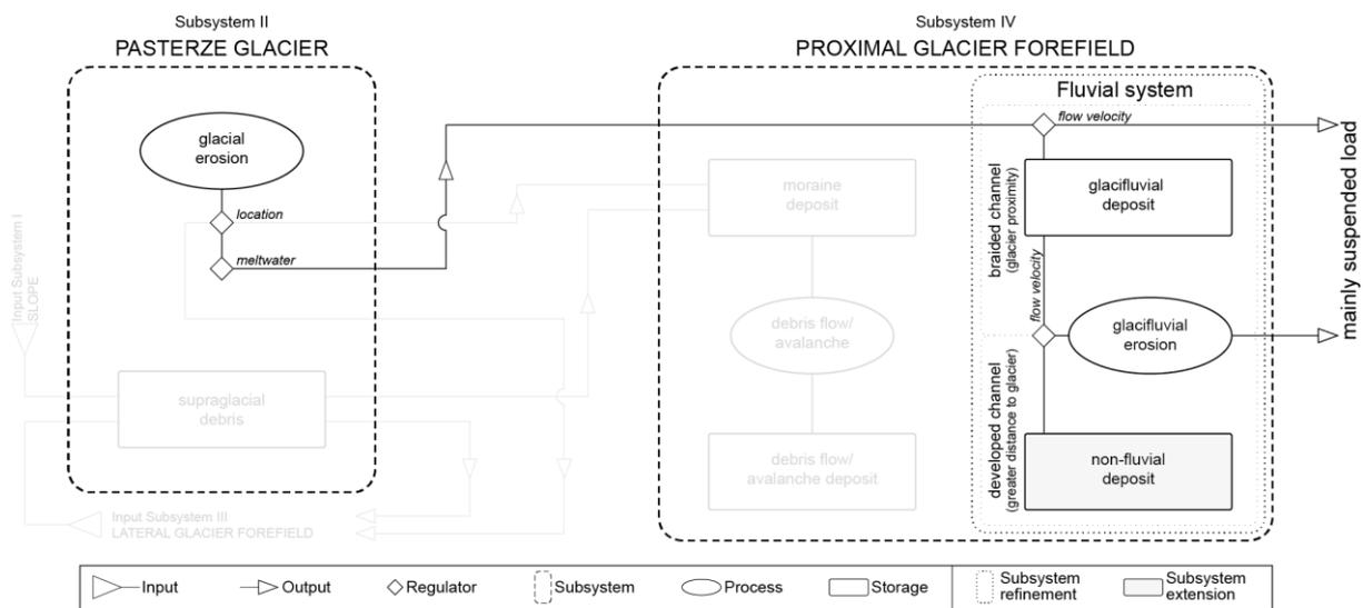
**Figure 19:** Refinement (dotted frames) and extension (grey highlighted in-stream sediment storage type) of the fluvial system within subsystem IV of the conceptual model of a sediment cascade for proglacial catchments. Due to the decoupled subsystems in the catchment (Geilhausen et al., 2012), the grey lines and connections only complete the cascade model but are irrelevant to the objectives of this study. Modified after Geilhausen et al. (2012).
