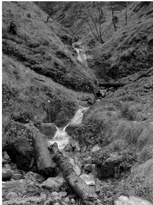
Figure 4: At LTER Zöbelboden, long-term physical and chemical runoff data is collected at measurement weirs (Foto: Umweltbundesamt).
